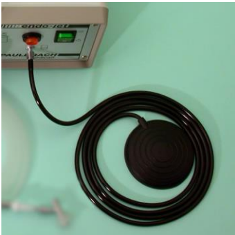
Figure 10: Connection to pneumatic foot switch
