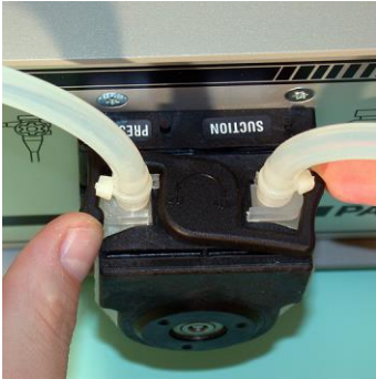
Figure 13: Unlock the sleeve
