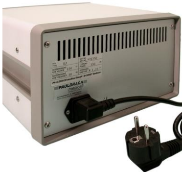
Figure 3: Plugging line cord
