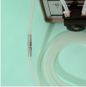
Figure 8: Connection of extension rinsing tube
