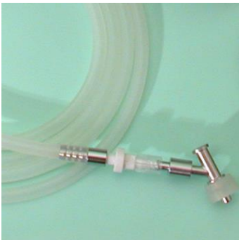
Figure 9: Connection to One-Way valve and ISA
